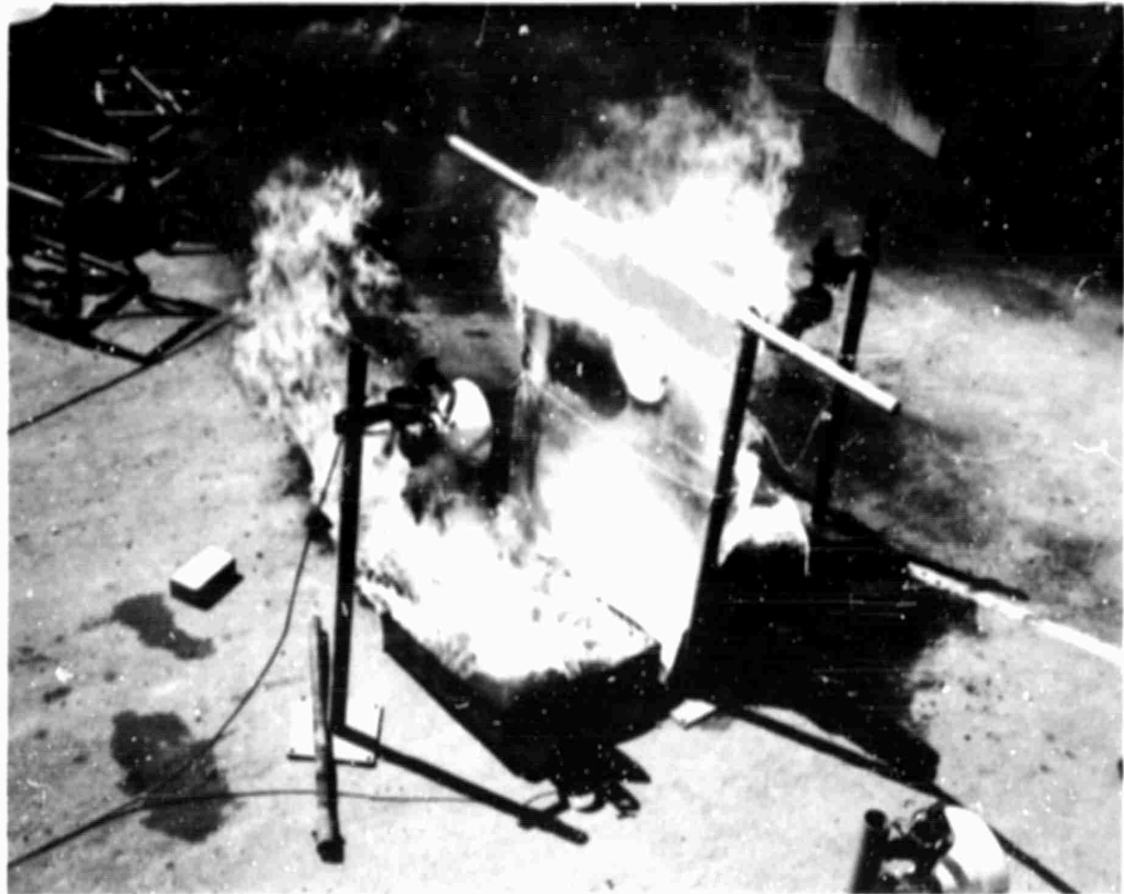
Figure 3.4 Sound velocity meter three feet above flaming gasoline. Asbestos baffle at midpoint of path.
