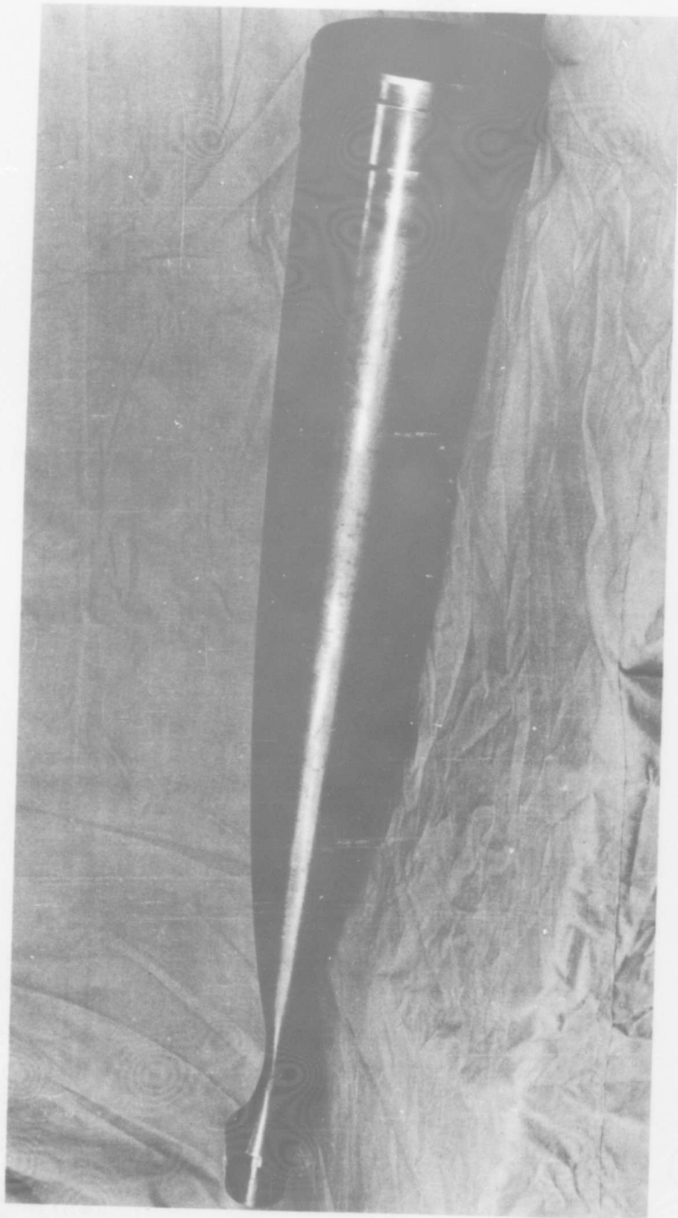
Fig.38 An electroformed nozzle liner (Sandberg-Serrell Corp.)
