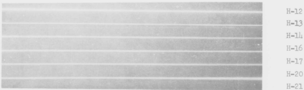
Figure 17. X-Ray Photograph: KT Silicon Carbide Test Bars, H-12 to H-14, H-16 to H-17, H-20 to H-21, 6" x 1/2" x 1/4" "As Fabricated", X-Ray through 1/2" Thickness
