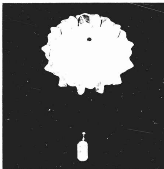
Figure 46 - Photograph of the personnel-type guide-surface parachute model (No. 26) during descent at approximately 20 feet per second.
