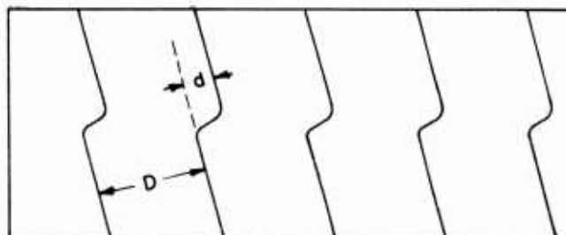
Figure III D-2 Fringe Pattern Showing the Effect Produced by the Step of the Thin Film
