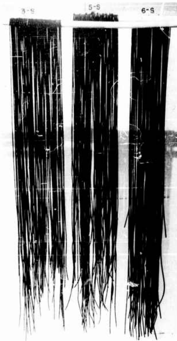
Figure 13. Comparison Of Three Modified Formulation Benite Lots For Straightness After Drying (Front View)
