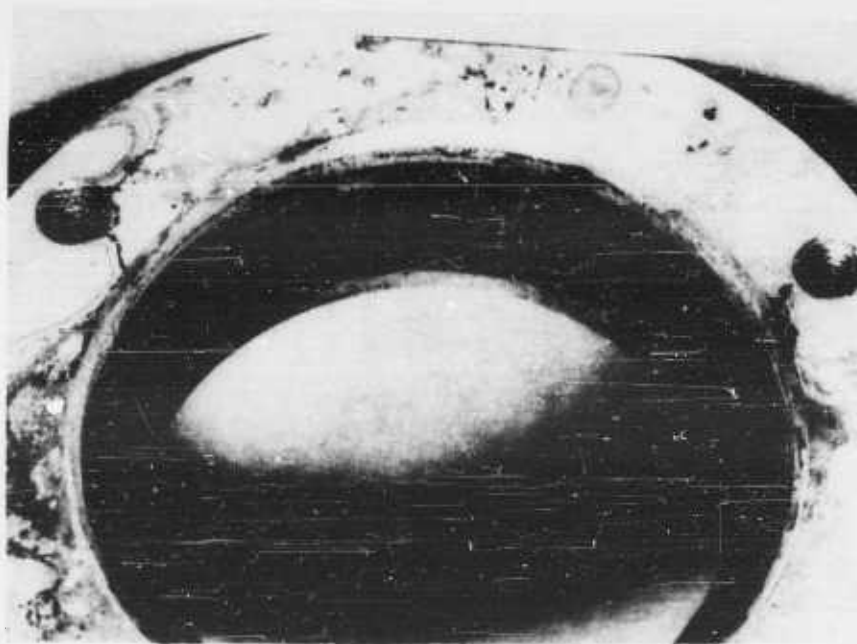
Figure 101. MCR 205-C Roller Bearing Outer Race - SAE 52100 Steel
