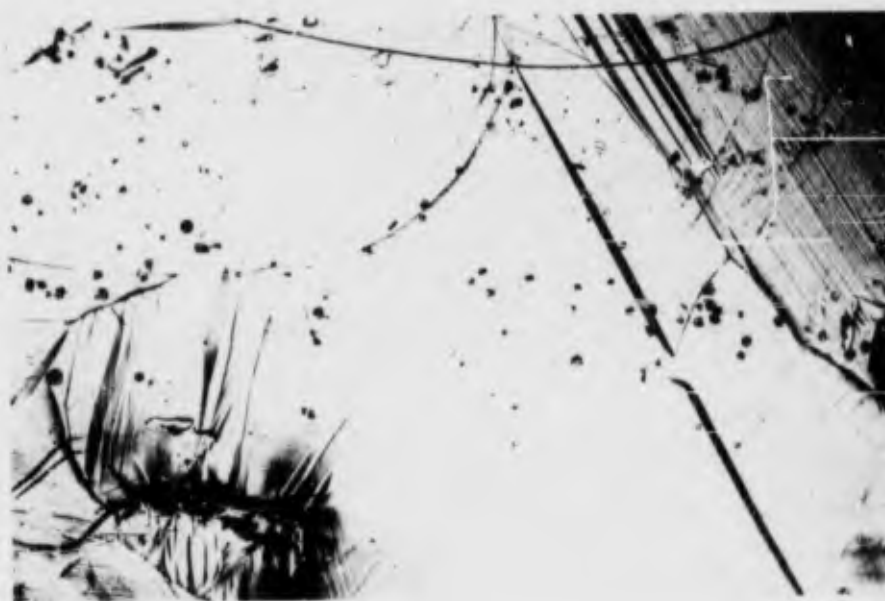
Fig. 9 Slip and twin traces in polycrystalline cadmium, tested in compression at -196^{\circ}\text{C} a) specimen Cd-S-12, 20 per cent strain, x50 b) specimen Cd-S-2, 15 per cent strain, x150
