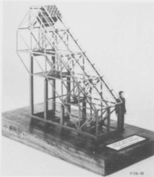
Fig. 71-1. Partial model of a typical phased-array antenna.
