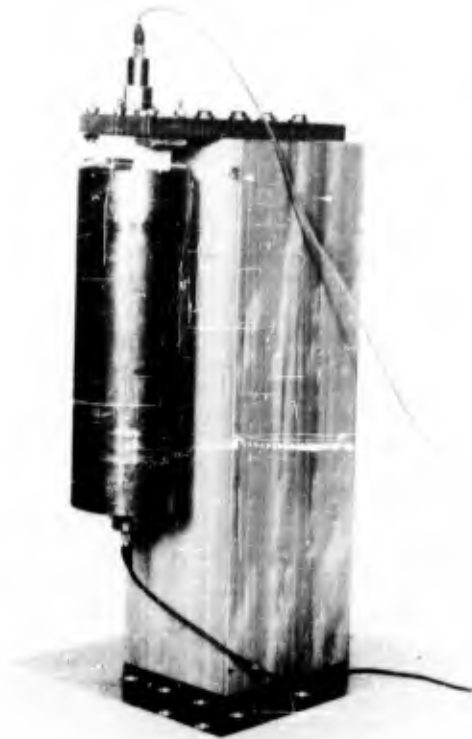
Fig. 6 - Vibration test fixture for coupled-compression isolator (aircraft type)
