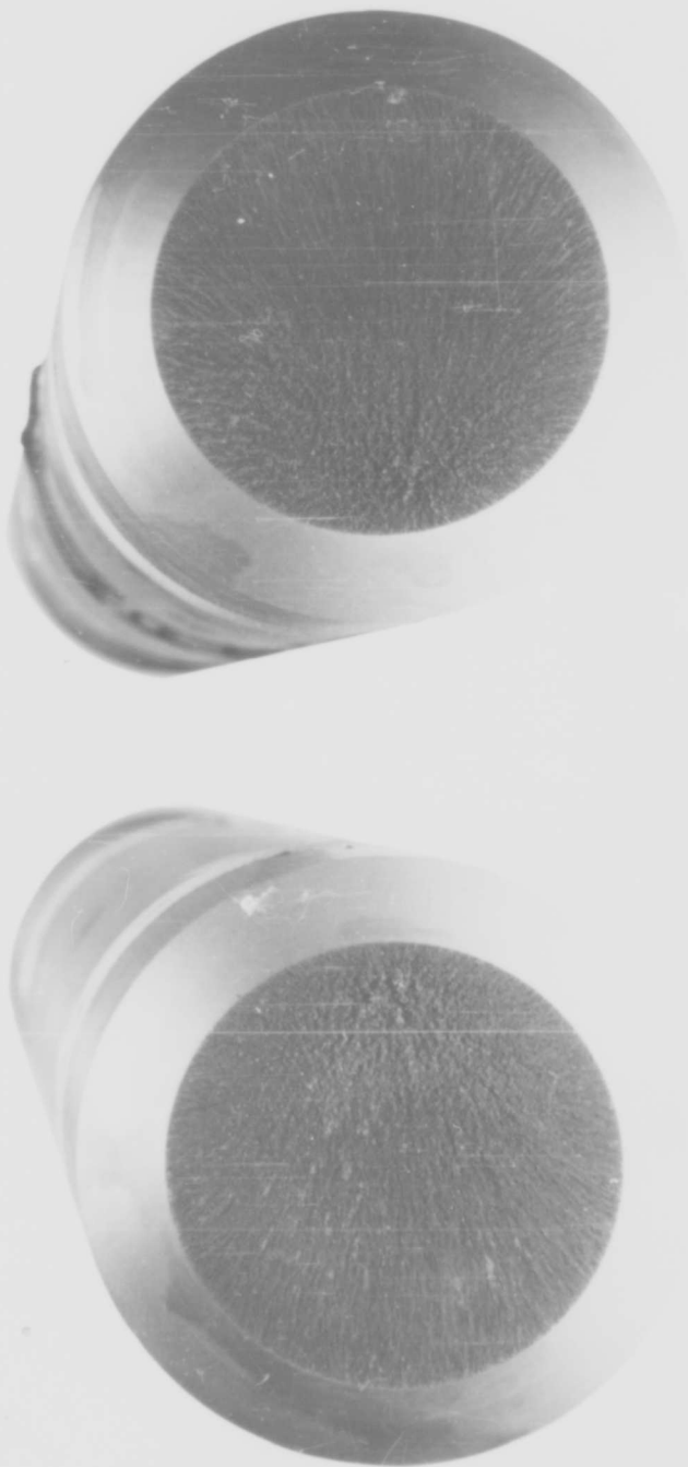
Figure 6. Fracture Appearance of 3 inch specimen of 4330V (Mod + S1) Steel Tempered at 600° F
