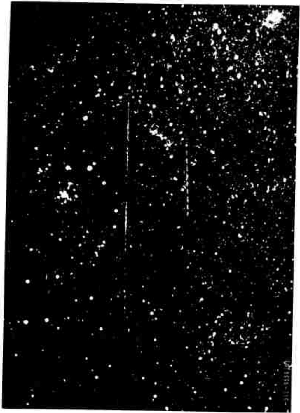
Fig. V-12(b). Eastville Super Schmidt photograph of Trailblazer Ig. Shorter trace is seventh stage. Camera and conditions as given for Fig. V-12(a) except for location and shutter rate of 15 breaks per second.
