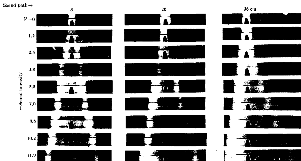
FIG. 2. "Narrow beam diffraction" by ultrasonic waves in water. F=1.76 Mc. W=\lambda/2 .
