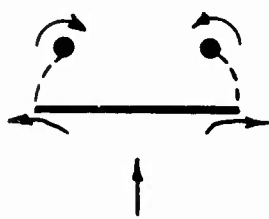
b. Edwards and Brown-and-Michael model for cross-flow plane of a slender delta wing
