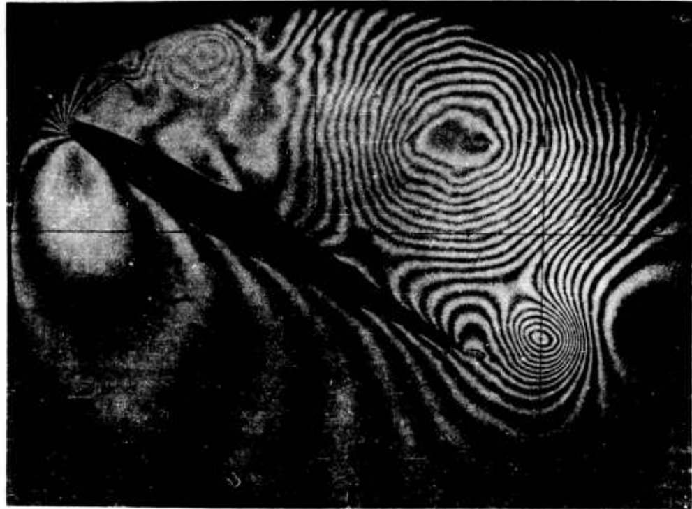
Fig. 11 Single-Fringe Interferogram of Formation of Second Trailing-Edge Vortex, NASA 64A010 Profile, \alpha = 30 deg., M_2 = 0.4 , \frac{M_2^2}{c} = 3.08 .
