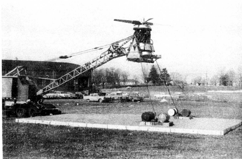
Figure 9: TEST SET-UP FOR OPERATIONS OVER SAND TERRAIN
