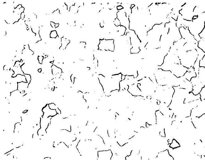
FIGURE 11 Ti-5Al-5Sn-5Zr, V-1540, 0.062in SHEET. HEAT-AFFECTED ZONE, WELDED + 1650F (1/2 hr) AC, SHOWING RECRYSTALLIZATION OF PARENT METAL AND HEAT-AFFECTED ZONE.
