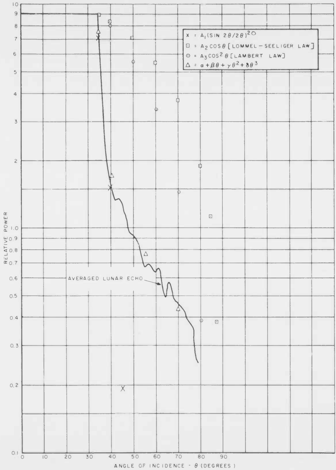
Figure 29. Scattering Laws Applied to Lunar Echo as a Function of the Angle of Incidence
