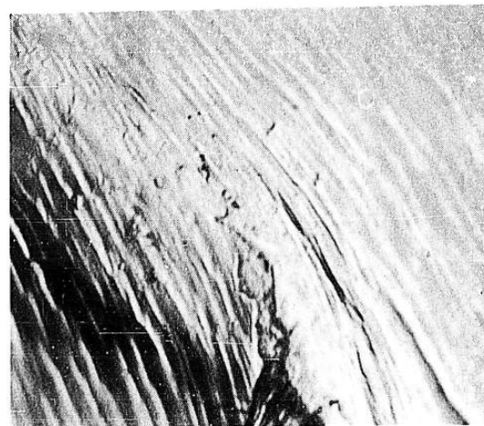
FIGURE 50. SHEAR FRACTURE IN STRESS-RELIEVED RHODIUM
