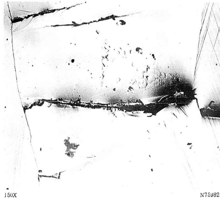
FIGURE 51e. SURFACE REPLICA AFTER ABOUT 2 PER CENT STRAIN IN COMPRESSION Oblique lighting.
