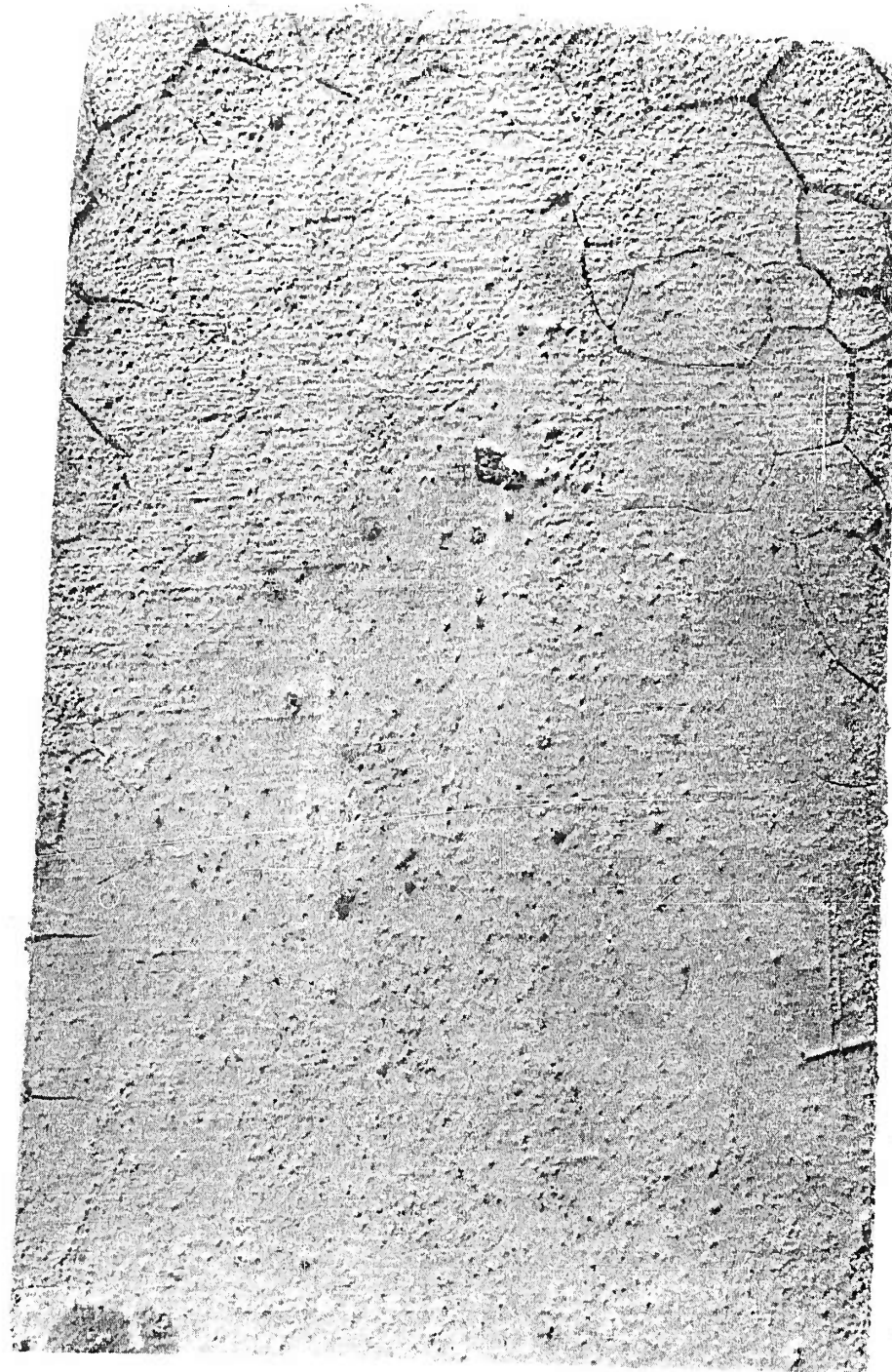
FIGURE 71. APPEARANCE OF RUTHENIUM AFTER OXIDATION AT 1200 C FOR 6 HOURS
