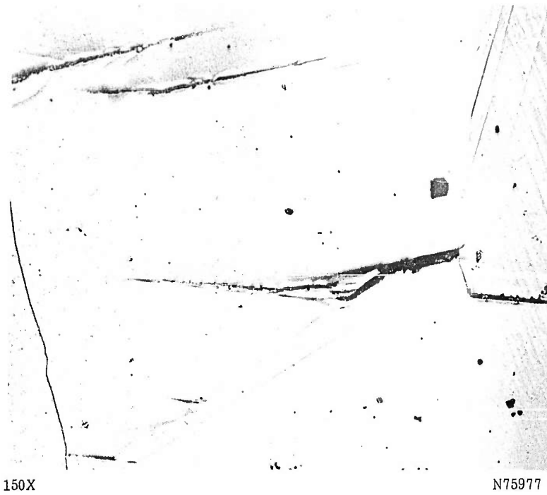
FIGURE 51c. SURFACE REPLICA AFTER ABOUT 0.8 PER CENT STRAIN IN COMPRESSION
