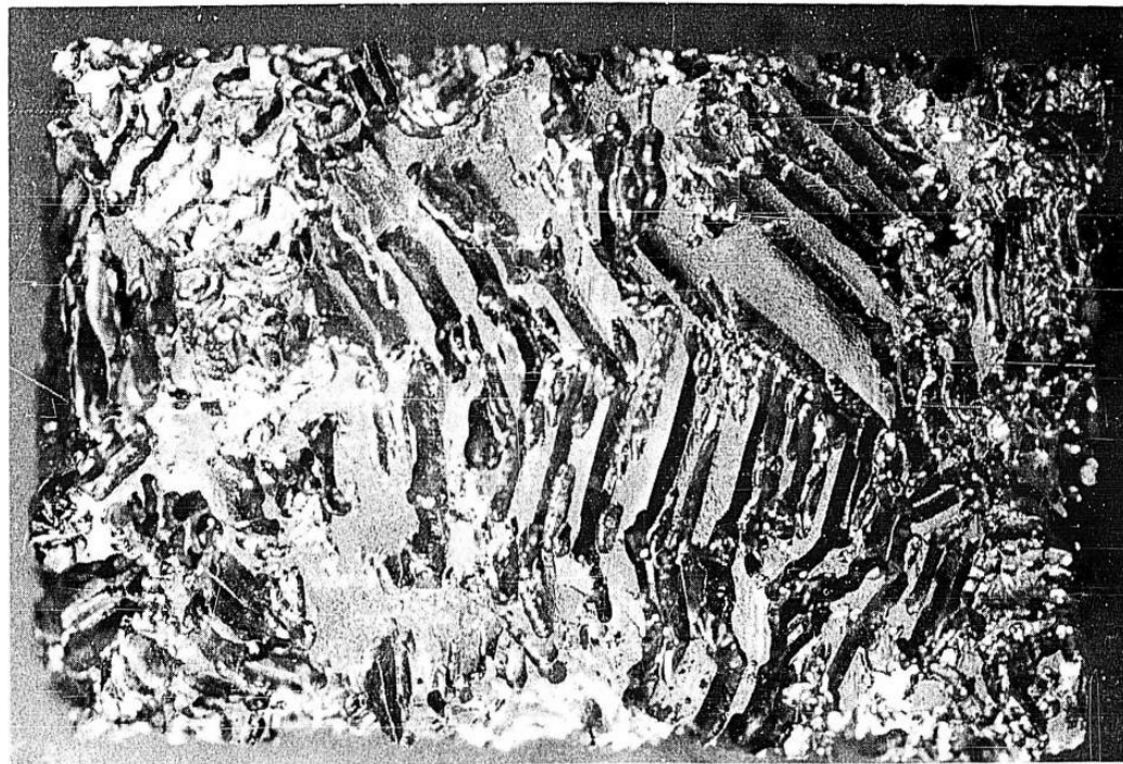
FIGURE 74. APPEARANCE OF OSMIUM AFTER OXIDATION AT 1400 C FOR 40 MINUTES
