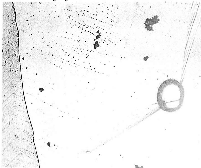
FIGURE 51b. SURFACE REPLICA AFTER ABOUT 0.2 PER CENT STRAIN IN COMPRESSION
