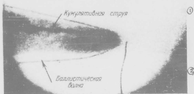
Fig. 172. Spark photograph of dispersed cumulative jet (45 microseconds after start of explosion).
