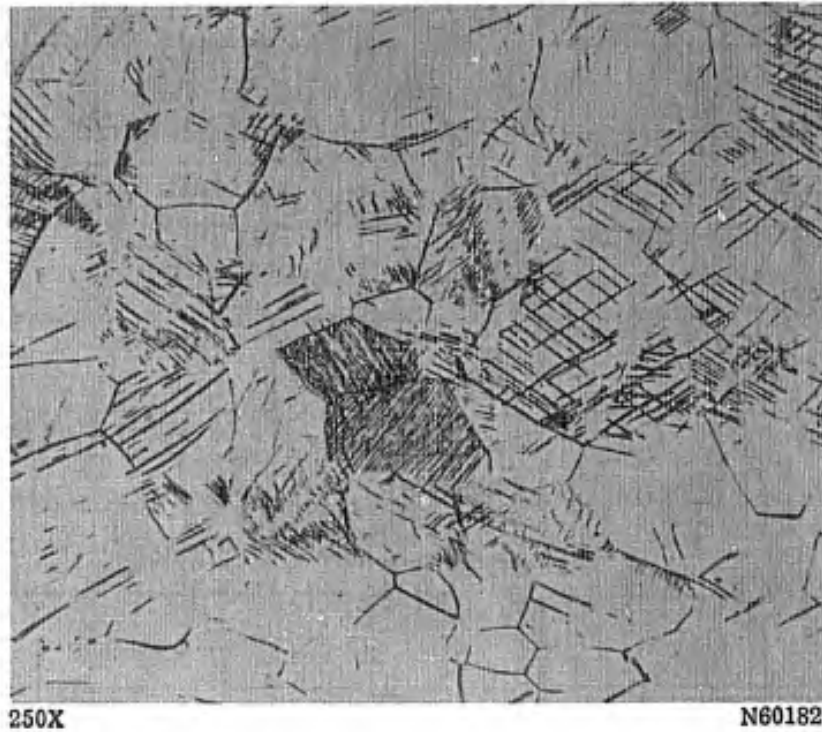
FIGURE 19. STRAINED PORTION OF ROOM-TEMPERATURE TENSILE SPECIMEN ON THE Ta-40Ti ALLOY
