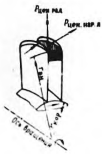
Fig. 1. Forces acting on the gas between turbine blades. a) P_{\text{cen.rad}} b) P_{\text{cen.nor.b}} c) r_{\text{ext}} d) r_{\text{cor}} e) rotation axis.
