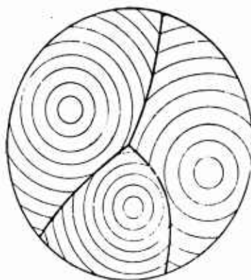
Fig. 90. Sketch of the formation of a joint of three grains with spherical syngony of the growth. Plane of the drawing runs through the center of the crystallization of the grain, rate of growth of which varies
