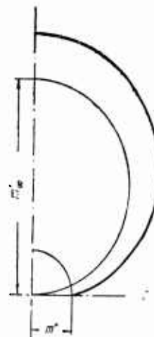
Fig. 63. Graphic construction of the plane rose of the number of intersections for the partially oriented system of lines in accordance with the the numbers of intersections on secants parallel and perpendicular to the axis of orientation.
