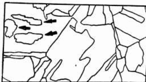
Fig.6 - Isolated Grains in Austenite Steel (18% Cr and 8% Ni) (Sibl.36)
