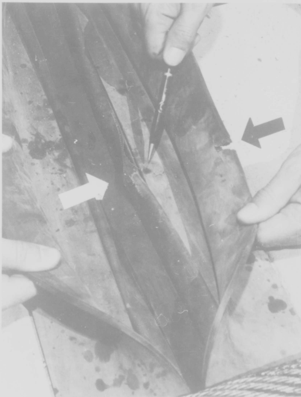
FIGURE 36: PINCH DAMAGE TO TROUGH UNIT
