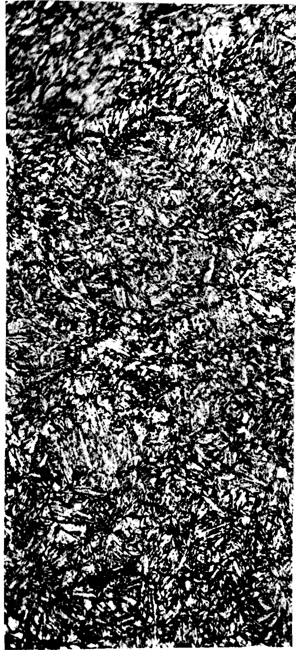
SERIES S AND E - TYPICAL MARTENSITIC MICROSTRUCTURES AT 1000X MAGNIFICATION
