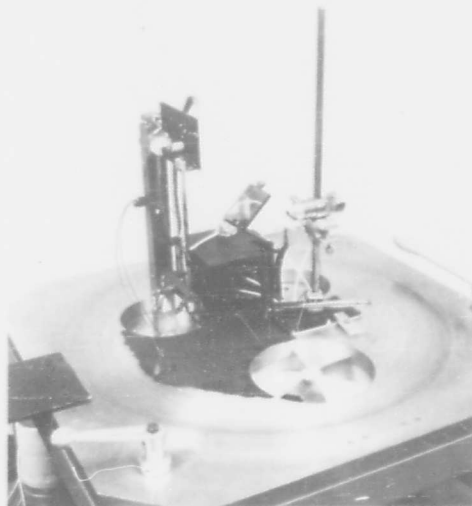
Fig. 5 Detail photograph of apparatus for measurement of time dependence of emittance.
