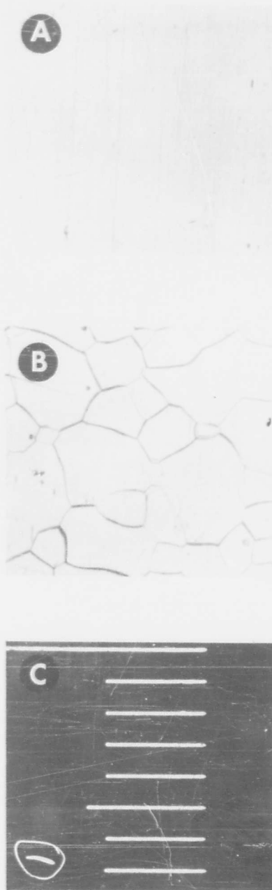
Fig. 22 Photomicrographs of the platinum surface: (a) as received, (b) after 4.5 hours at \approx 1500^{\circ}\text{K} , (c) scale with 100 micron separation between marks.
