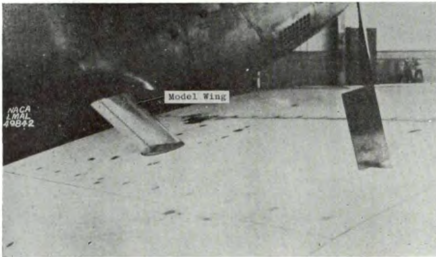
FIG. 2.10. Wing-flow method demonstrated by model mounted on wing of P-51D airplane (1947). A
