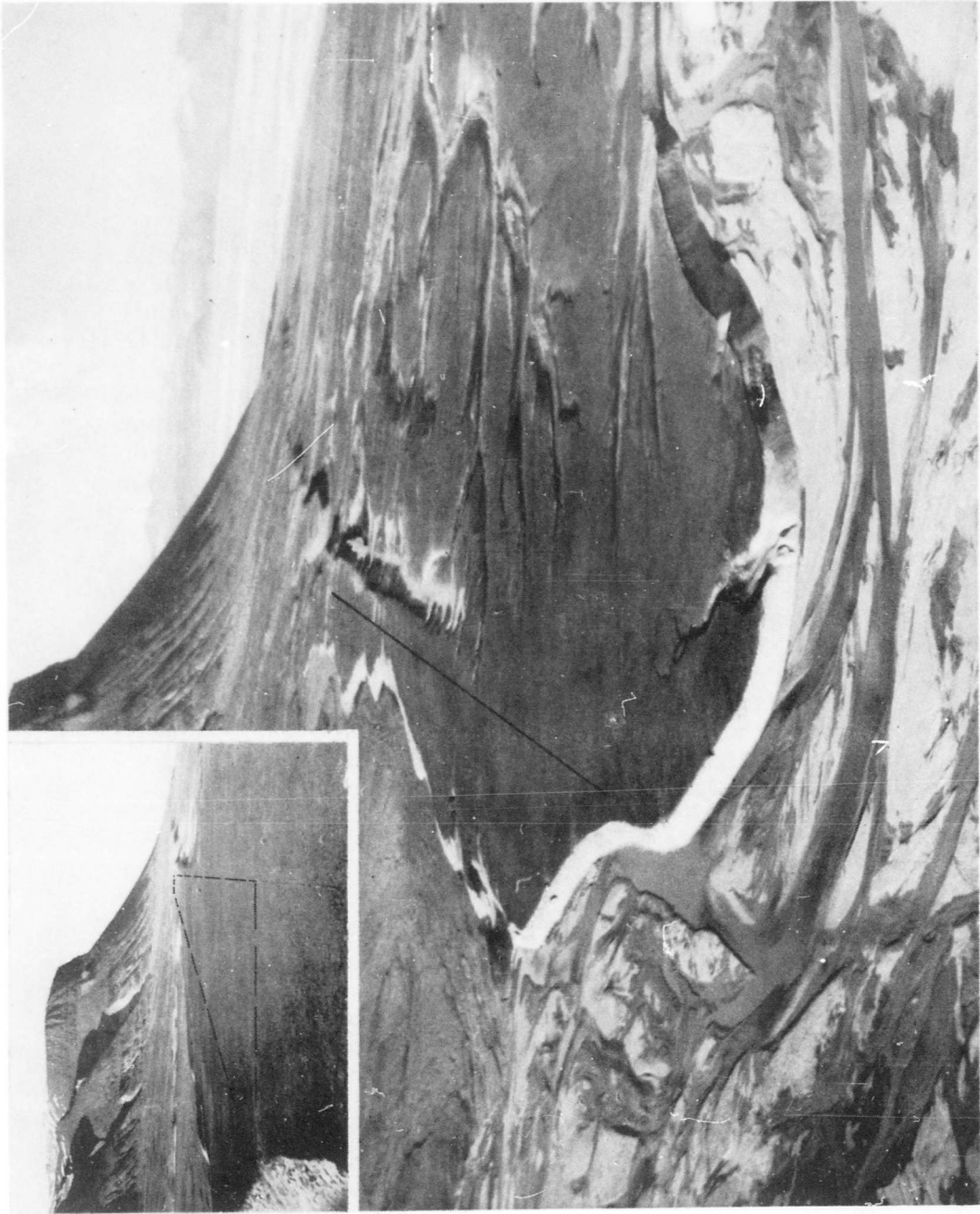
Photograph 5. Aerial views of the Carlsberg Fjord Site (#10), looking northward along a ridge of dissected valley fill, perhaps outwash gravel, located in valley on west side of Carlsberg Fjord. Centerline and outline of a potential 4000-foot runway are shown, oriented approximately N30° E. Date: 27 August 1959.
