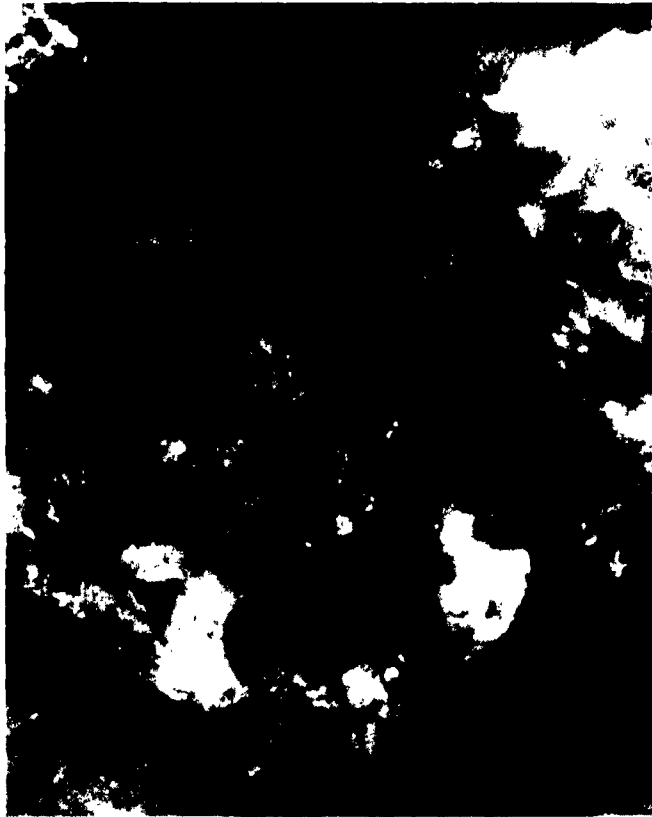
Fig. 23 - Transformation of structure in the negative plate to coarse particles is illustrated when the conditions were as in Fig. 22 except that the specific gravity of electrolyte was increased to 1.45. A tendency for some of the lead sulfate particles in the upper part of the picture to appear somewhat translucent will be noted. 1000X magnification.
