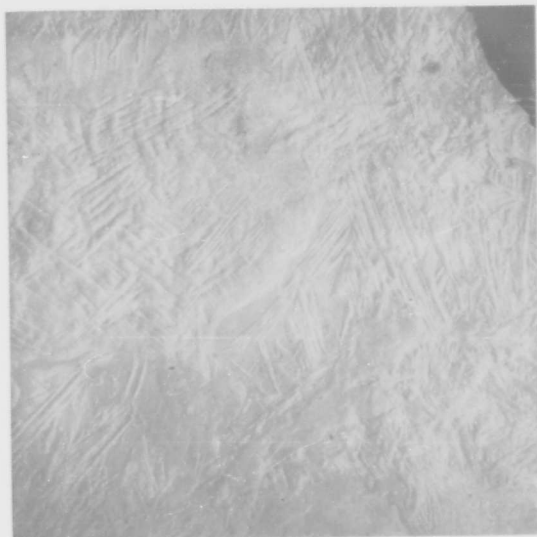
Fig. 19 a. Electron micrograph (replica) of surface of coldrolled Ta-specimen (polished and etched before oxidation) oxidized for 300 min. at 500° C and 10 torr oxygen. 3550 x.
