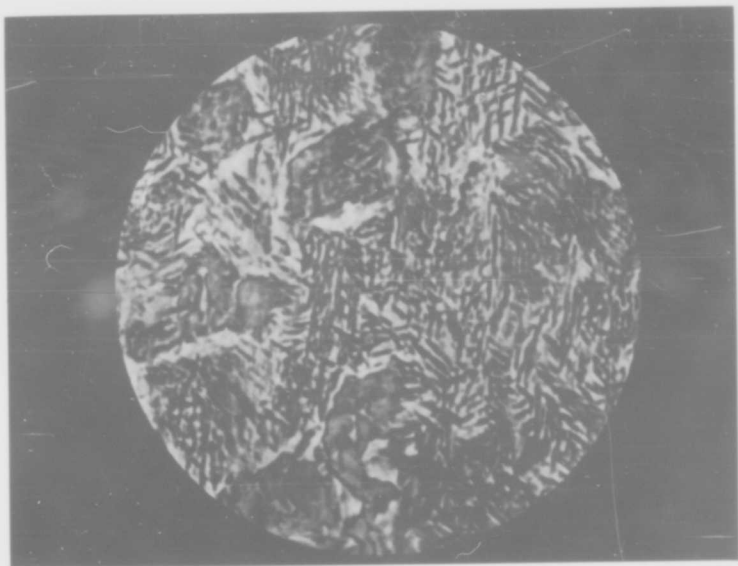
Fig. 9. Surface of cold-rolled Ta-specimen oxidized for 3200 min. at 350° C and 1 atm. oxygen. 1750 x.
