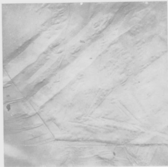
Fig. 19 b. Electron micrograph (replica) of surface of high vacuum annealed Ta-specimen (polished and etched before oxidation) oxidized for 300 min. at 500° C and 10 torr oxygen. 3550 x.
