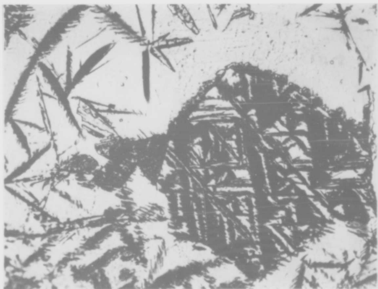
Fig. 12 b. Surface of high-vacuum annealed Ta-specimen oxidized for 300 min. at 500° C and 10 torr oxygen. 500 x.
