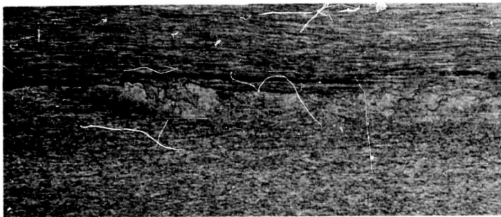
B. Tungsten (0.030-inch) Mo-0.5Ti (0.032-inch) (40X)
