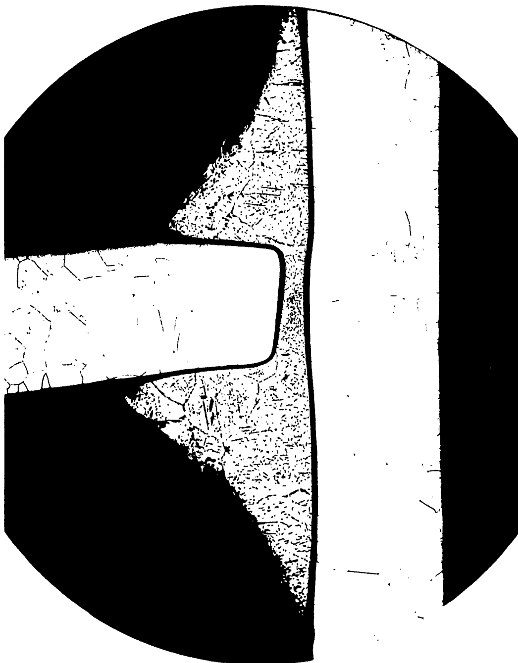
A photomicrograph of a D-36 T-joint brazed with commercially pure titanium at 3100° F. Filletting action of the braze alloy is marginal at this temperature. (75x)
