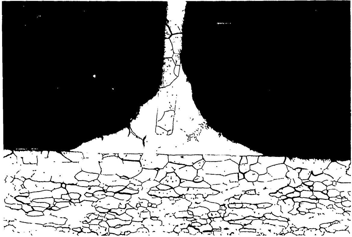
A photomicrograph of a typical TzM core to skin fillet brazed with commercially pure titanium at 3100° F. (200x)
