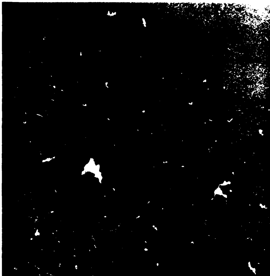
Fig. 8. Electron Micrograph of Cabot \text{Al}_2\text{O}_3 powder (direct carbon replica preshadowed with platinum metal).
