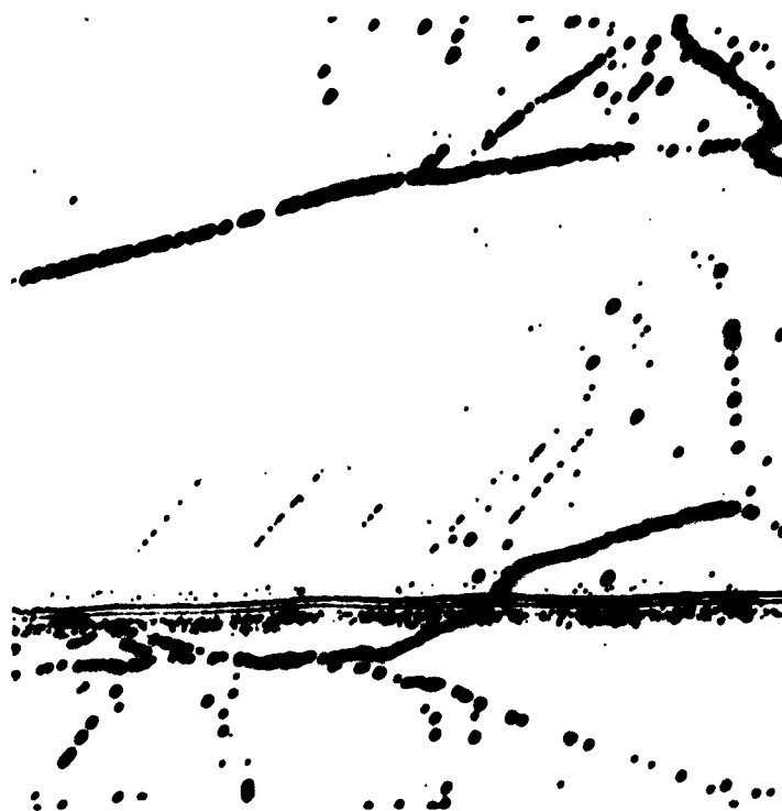
Fig. 54 Dislocation motion from a scratch in tungsten, 250X. (a) Crystal stressed at 77°K; (b) crystal stressed at 298°K. Difference in number of dislocations moving from the scratch is the result of both temperature and applied stress.
