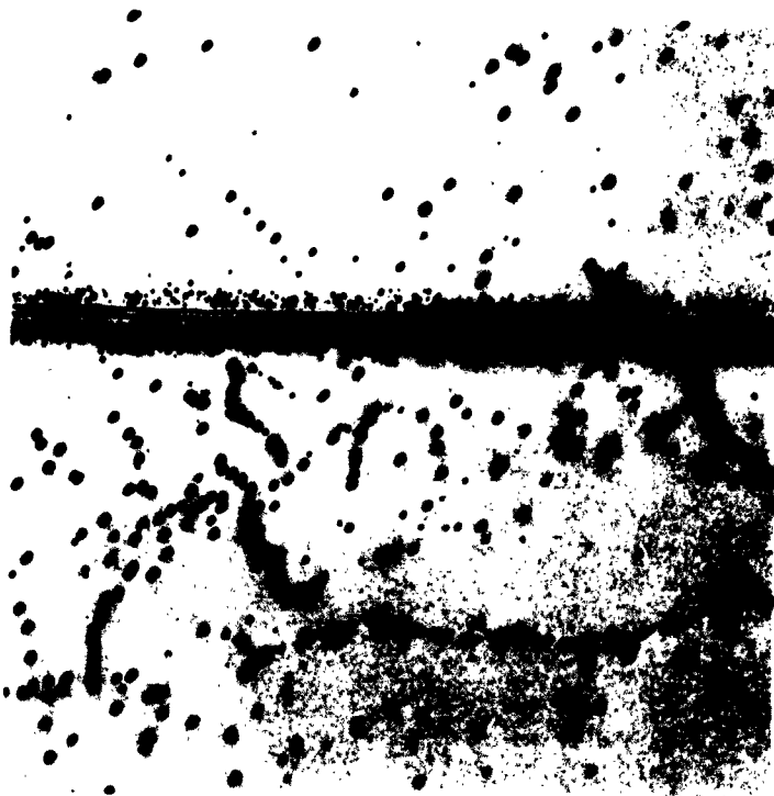
Fig. 51 Character of scratch formed on (112) type surface of tungsten crystal scratched at 77^\circ\text{K} . 250X
