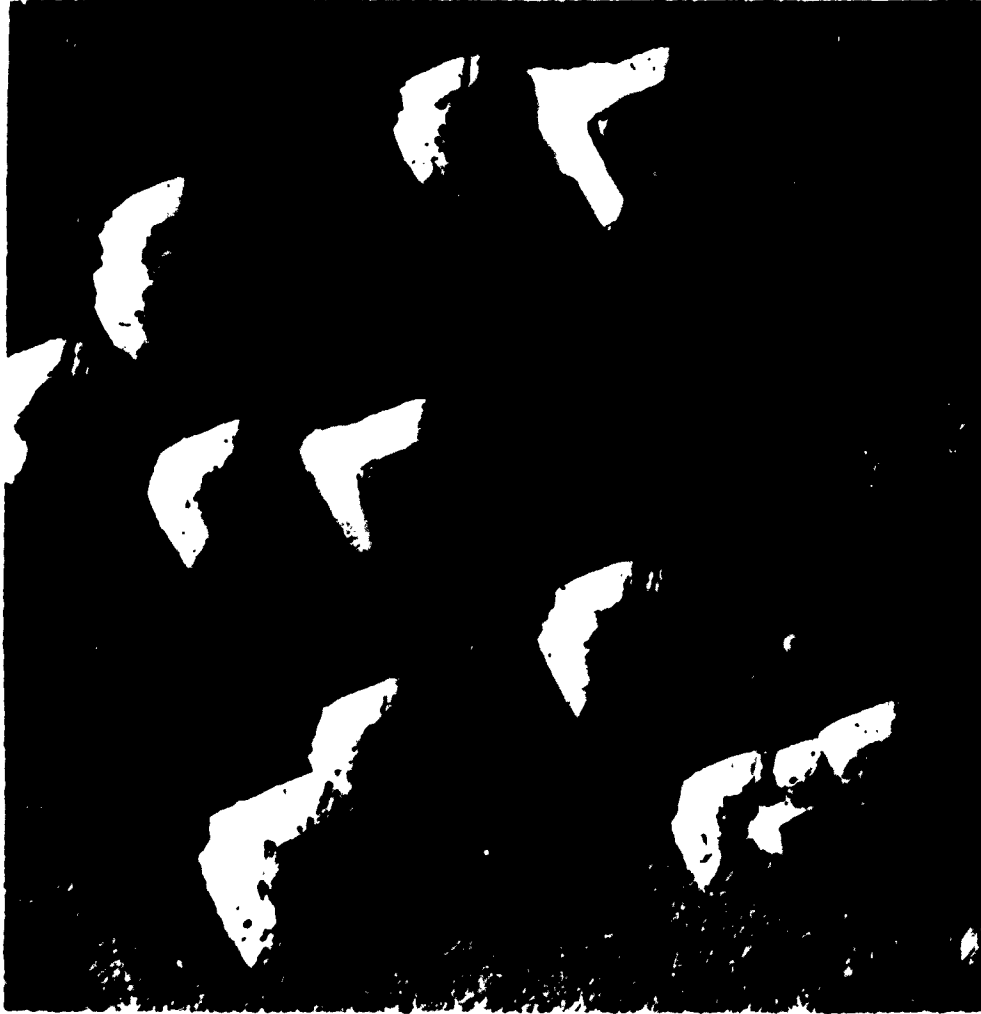
Fig. 24 Electron microscope picture of pits formed \{100\} surface of tungsten crystal. 10,000X
