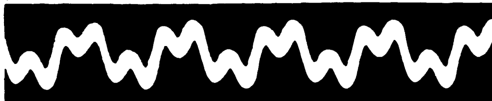
Figure 8. Streak Record of X26 Crystal Response to 1150 cps Square-Wave Excitation
