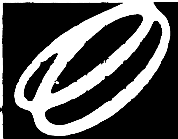
Figure 7b. Response of X26 Resonant-Modified Crystal Transducers - Major Axis: 3450 cps, 150 V rms - Minor Axis: 3450 cps, 100 V rms, 90^\circ \phi , Plus 1725 cps, 50 V rms
