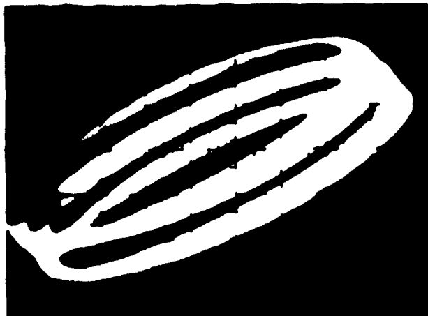
Figure 7a. Response of X26 Resonant-Modified Crystal Transducers - Major Axis: 3450 cps, 150 V rms - Minor Axis: 3450 cps, 100 V rms, 90^\circ \phi , Plus 862.5 cps, 50 V rms
