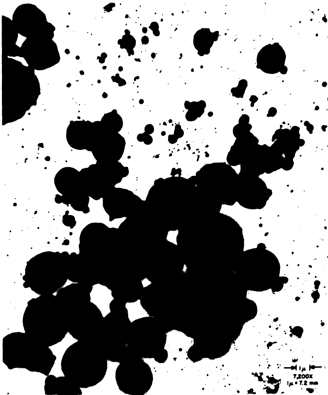
Fig. 7. Micrograph of aluminum oxide sample obtained from motor firing at 500-psi chamber pressure
