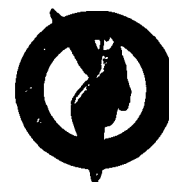
MAG: 5X GAGE AREA SURFACE OF FAILED CYCLIC TEST SPECIMEN NO. 7 TIG-WELDED IN THREE PASSES (V-TYPE PREPARED JOINT). SPECIMEN FAILED AT 170,000 PSI THROUGH PRIOR CRACK NOT ASSOCIATED WITH WELD POROSITY. NOTE DISCONTINUITY IN WELD BEAD AT FRACTURE
