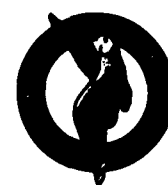
ETCHANT: 5% HF, 35% HNO 3 MAG: 2X MACROSTRUCTURE OF RADIAL SECTION THROUGH HALF SECTION OF POLAR BOSS FROM FULL SCALE 40-INCH DIAMETER FRONT DOME ELA-3 PRESS- FORGED AT 1850F BY THE PANCAKE AND PREFORM METHOD. NOTE RELATIVELY FINE BUT EQUI-AXED GRAIN STRUCTURE WITH SOME COARSENING TOWARD INSIDE SURFACE (BOTTOM) H-25656
