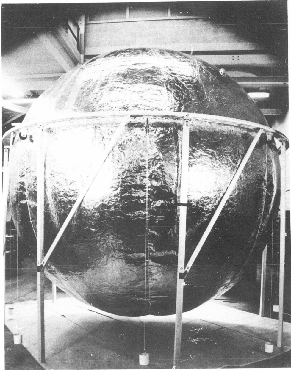
Figure 5.- Photograph of the testing of a 12-foot-diameter inflatable sphere.
