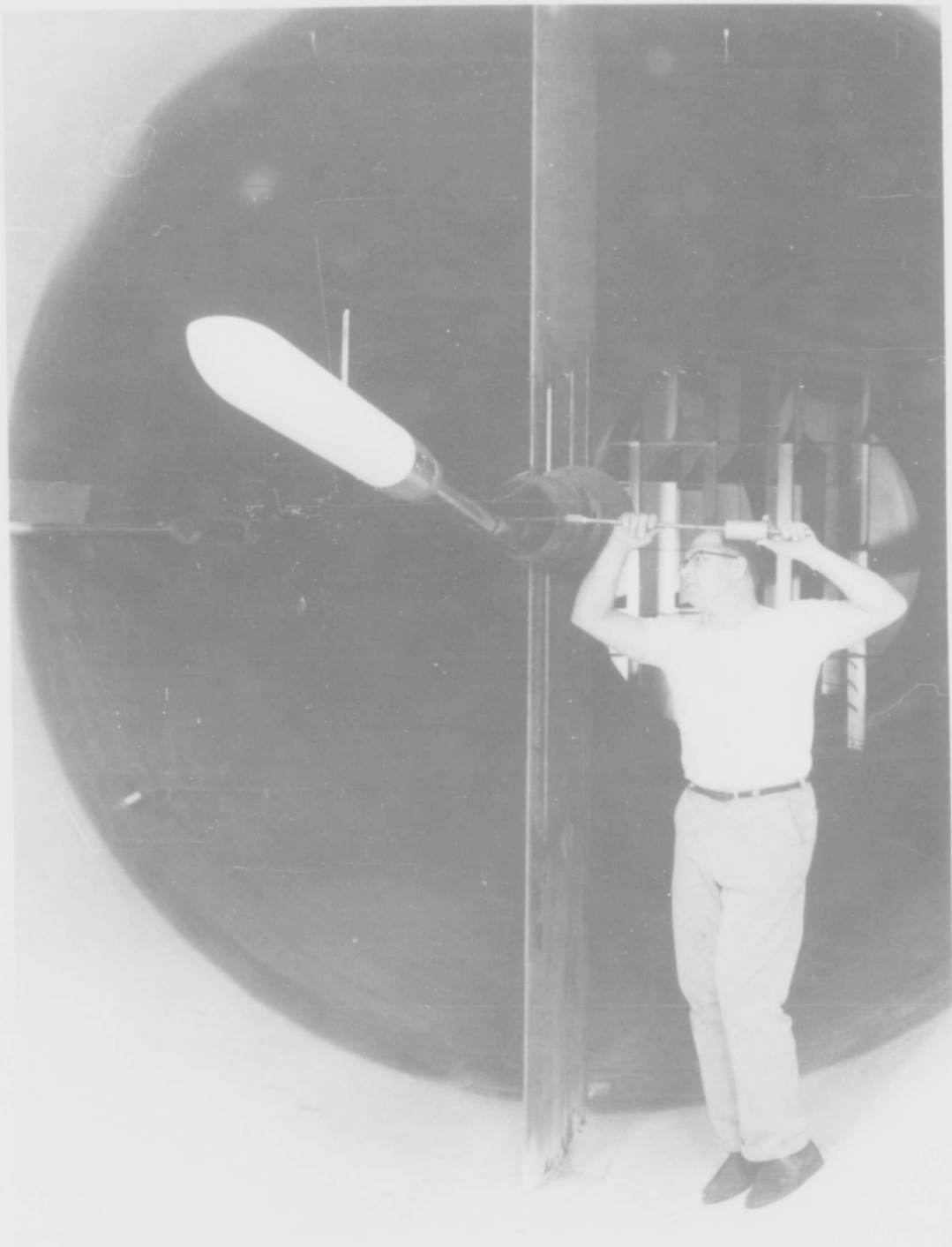
Figure 2.- The ogive-cylinder body of revolution in the wind tunnel.
