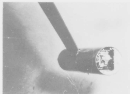
c. Base Ejection Installation Looking Upstream in the 50-in. Mach 8 Tunnel
