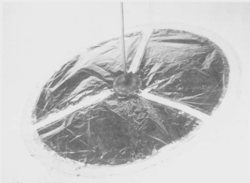
Figure 26. Inflated Torus-Sail Model
