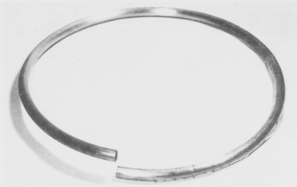
Figure 25. Segmented-Section Technique for Forming A Mylar Torus
