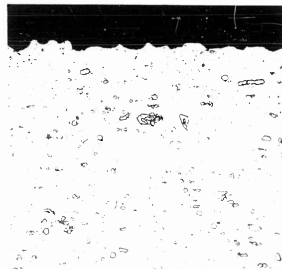
Figure 6. Surface Attack by 70% Nitric Acid on 2014 Aluminum Alloy when Exposed to Nitrogen in a Closed Flask (Magnification 500X)
