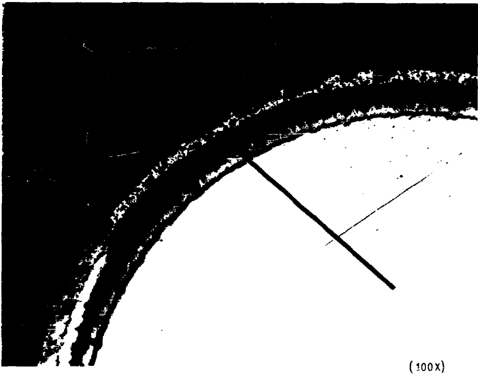
FIGURE 7. PHOTOMICROGRAPH OF LEAK PATH CROSS SECTION, SHOWING POROUS BRAZE
