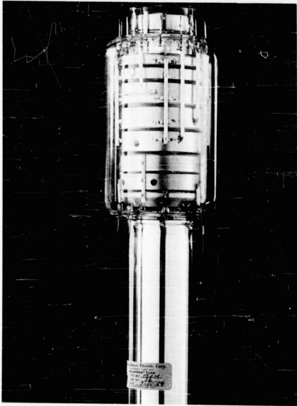
Figure 36. Image Orthicon with two TSEM Stages
