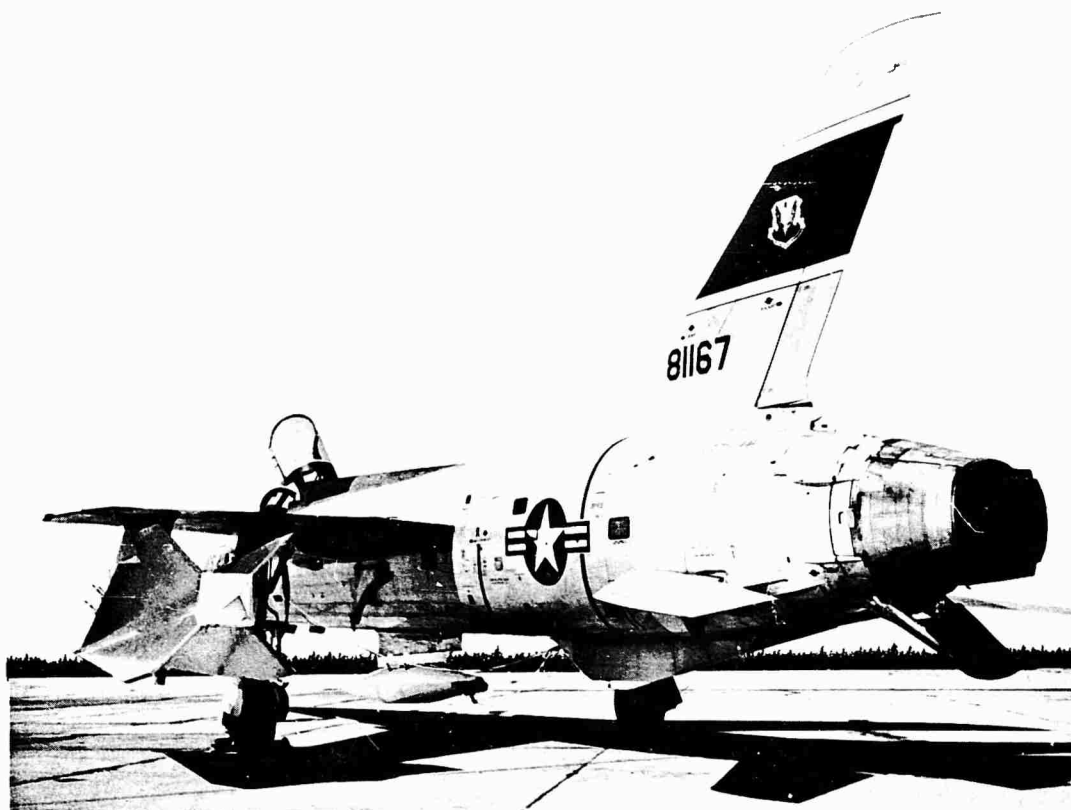
Fig. 1: Front and Rear Diagonal Views of F-105 Aircraft Showing Tow Target System Installation: (1) Centerline Pylon Adapter, (2) Tow Reel Assembly, (3) Parachute Recovery Canister, (4) Target Pylon Adapter, (5) TDU-10/B Target.
