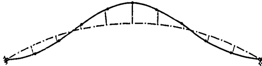
First Symmetrical Mode; \omega = 66.63 \sqrt{\frac{EI}{\mu L_0^4}}
