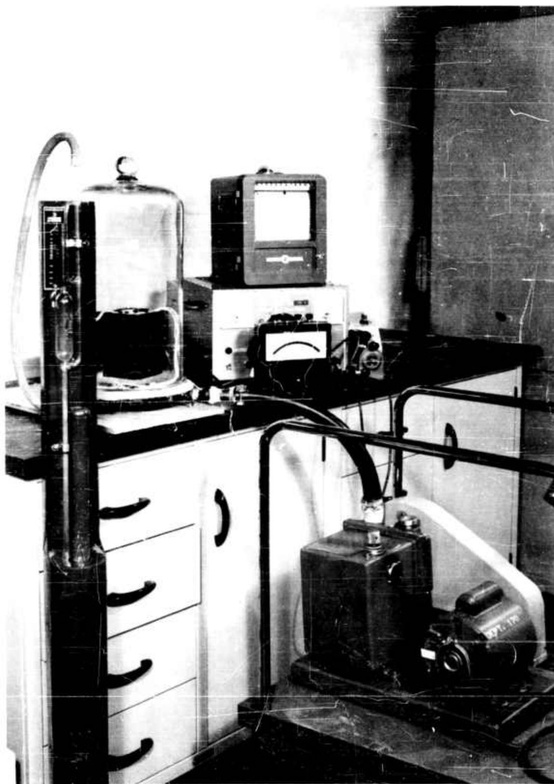
FIGURE 45 PRESSURE TEST OF 3-SEALED CELLS
