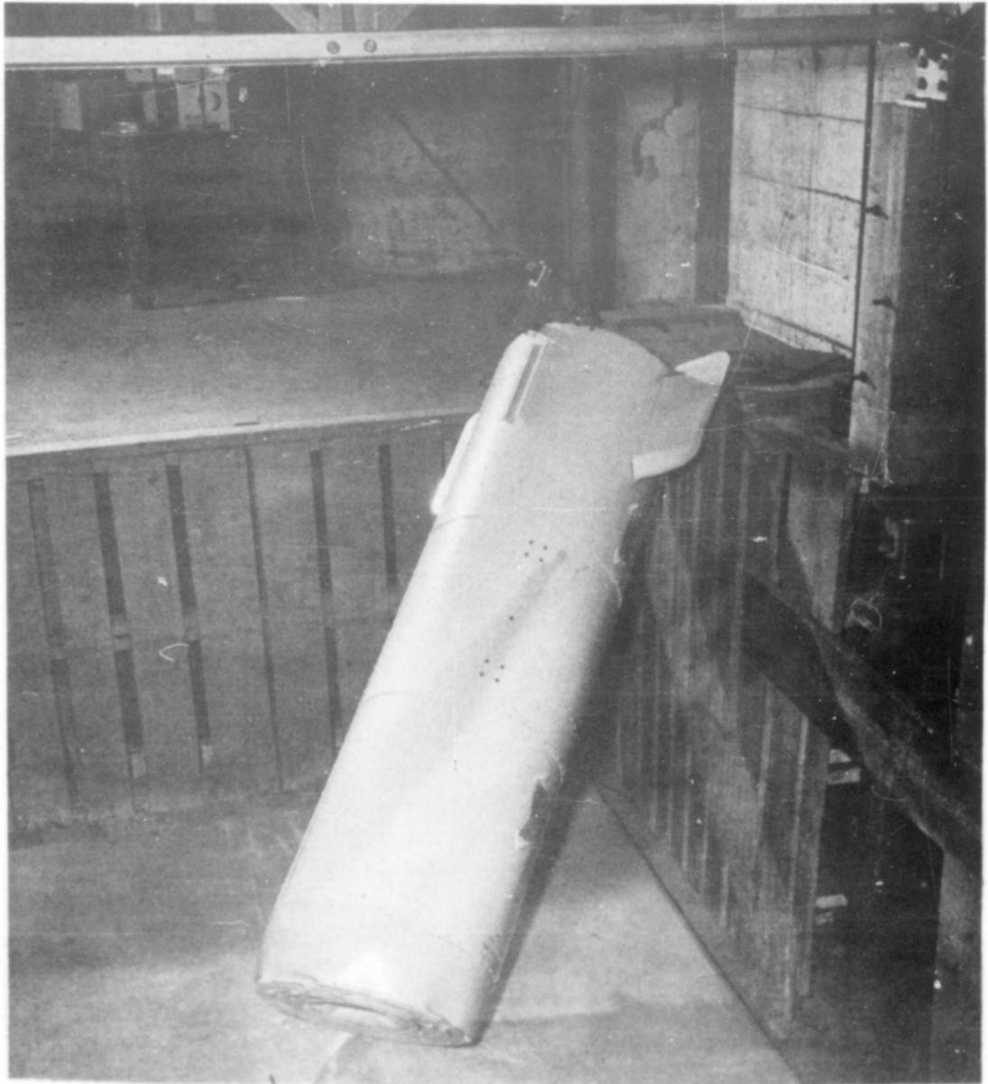
Figure 7. M-4A Container After Impact at 35 feet per second
