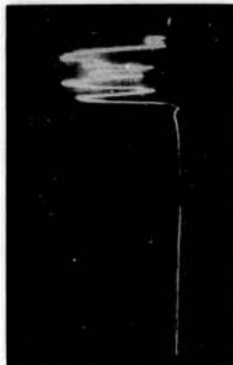
Fig. 25 Group of waves due to turbulence. Time constant: 1.5 msec, negative half-waves reversed
