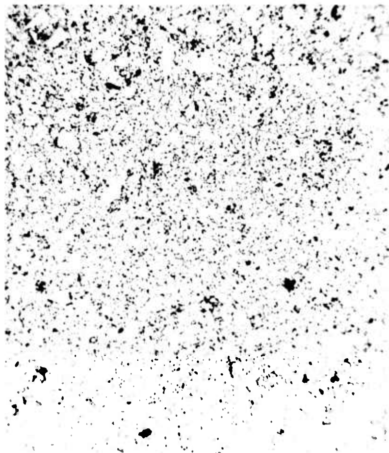
Figure 28 - Unfired Zirconium Carbide (Armour), Density 6.04 g/cc, etched X150
