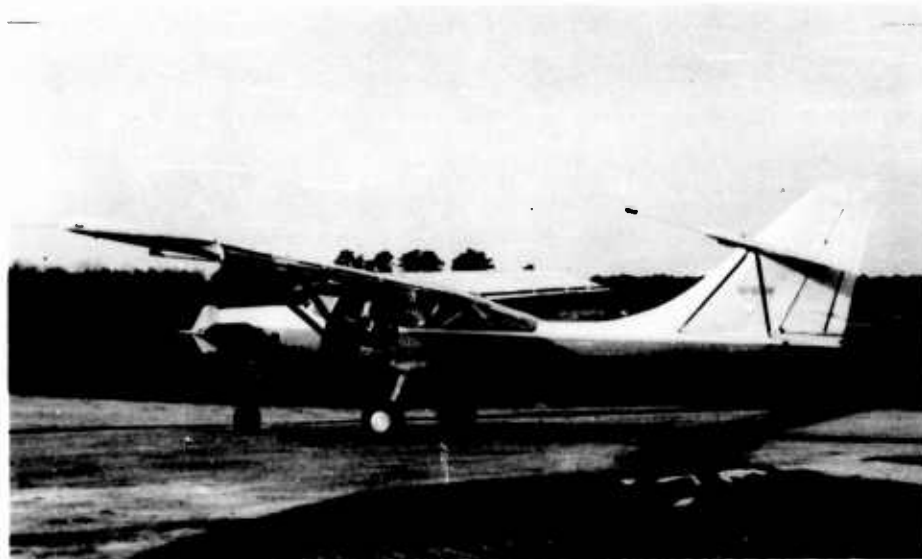
Figure 2. Robertson SKYSHARK Test Aircraft Equipped With U. L. S. ; Flaps and Shrouds Retracted.
